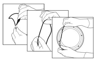
a. Lightly apply O-ring lubricant to the O-ring. Install the O-ring in the groove on the trim ring of the lower dome.
